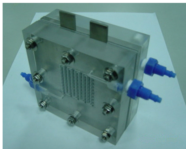
Fig. 3. A single-cell DMFC test fixture.
